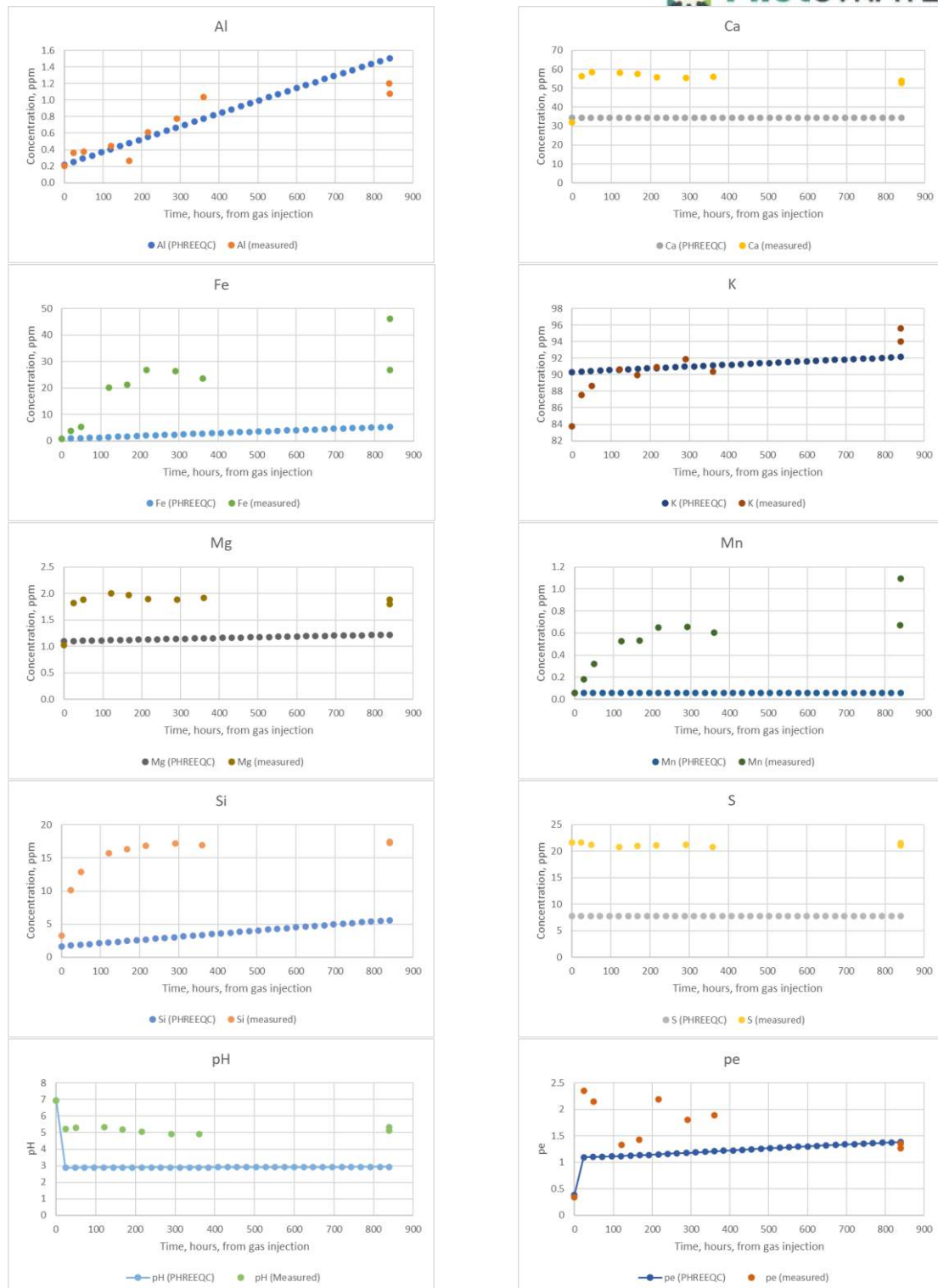
Figure 5.2: Modelled and measured fluid chemistry for reservoir sample experiment with CO 2 .
