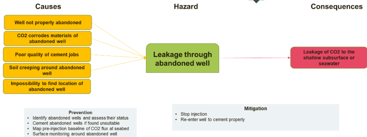
Figure 14: Bow-tie diagram to identify key causes, preventive barriers, potential consequences, and mitigation measures for the risk of leakage through an abandoned well.
