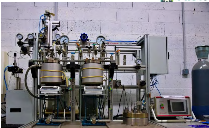
Figure 4-21. Picture of the TransREP experimental setup, part of the BioREP platform.
