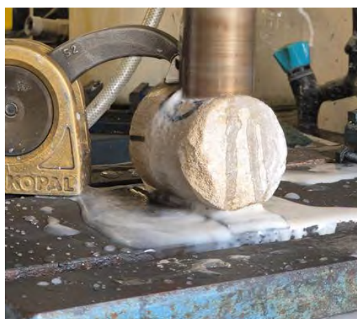
Figure 5-1: Transverse drilling of the SEIF-1 core in the representative core section of the Oolithe Blanche Formation
