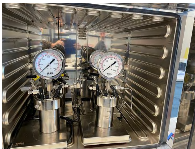
Figure 4-2 (below). Parr reaction vessels in oven, with magnetic stirrers and gas lines attached
