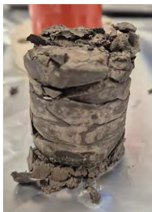
Figure 5-15: Photograph of the core plug SEIF 1 – 1841 after the end of the reactive flow-through experiment with CO 2 -enriched fluid (28 days).
