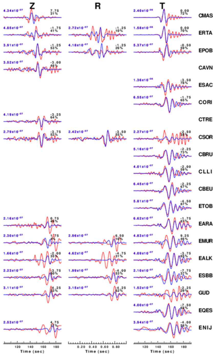
Figure 14. Comparison between the observed seismograms (red lines) and synthetic seismograms (blue lines) for solution obtained for the event. Left column = vertical component, center column = radial component, right column = transverse component. Each line of the seismograms corresponds to a seismic station, with its station code indicated to the right. The bottom scales are time in seconds.
