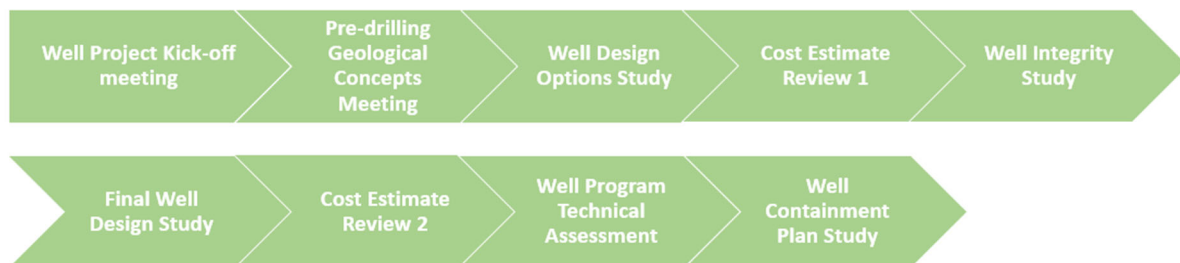
Figure 2.1: Well construction workflow proposal.
