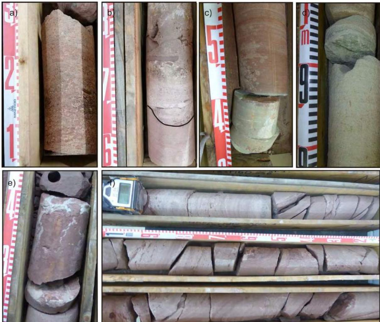
*Figure 9-72 Chiprana borehole. a and b) Cross-bedding sandstone with clay chips to bottom of Unit B1; c and d) intervals of siltstone and very fine to fine grained sandstones, planar, ripple and wave-ripple laminations of the Unit 1B; e) silts with nodules of carbonate; f) Cross-bedding sandstone with clay chips to bottom of Unit B2.*
