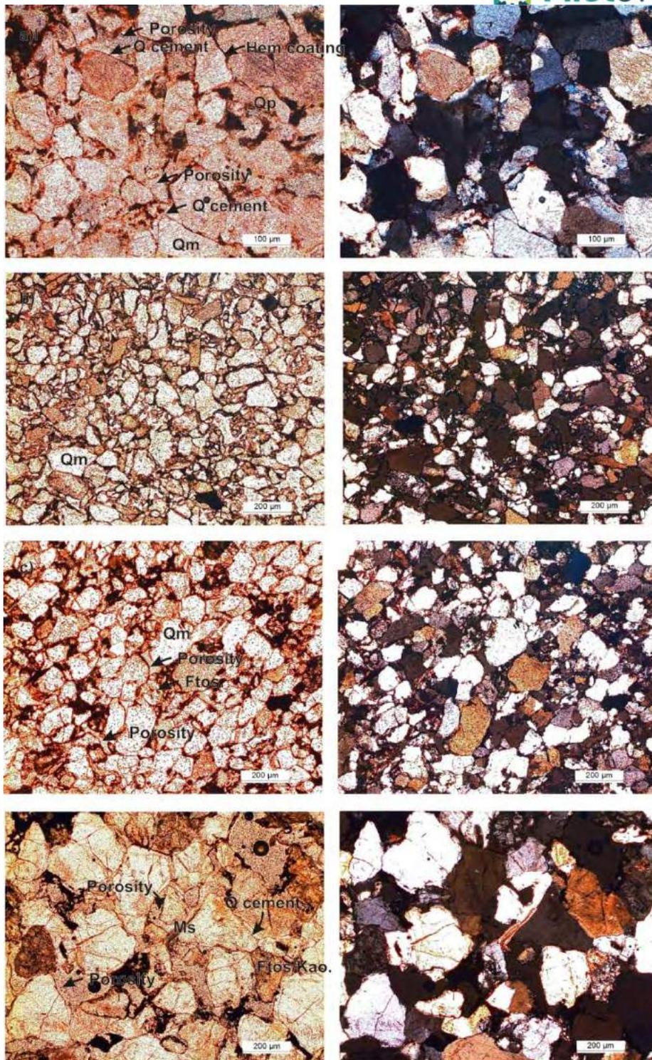
Figure 9-71 Representative microphotographs of thin sections (parallel and crossed nicols). a) Cross-bedding sandstone, bottom of Unit B1; b) Interstratification of ripple; c) Cross-bedding sandstone, top of Unit B1; and d) Cross-bedding sandstone, top of Unit B2.
