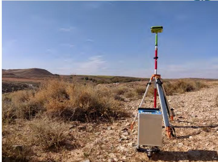
Picture 1. Example of gravimetry and GPS measurement.
